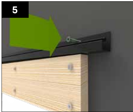
Fit the soaker trim to the wall at a slight angle, giving it a roughly one-degree fall. The battens should terminate above and below this trim.
